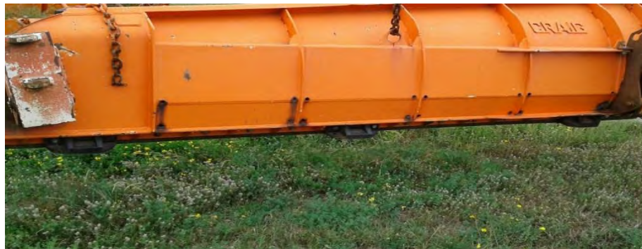
Note 3 Wing Shoes Installed On Back Of Wing, 1 Near Front, 1 Center, 1 Rear
