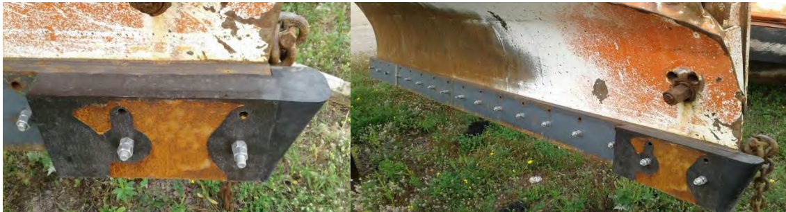
Pictured above is a front rubber wing block installed on a Craig wing
